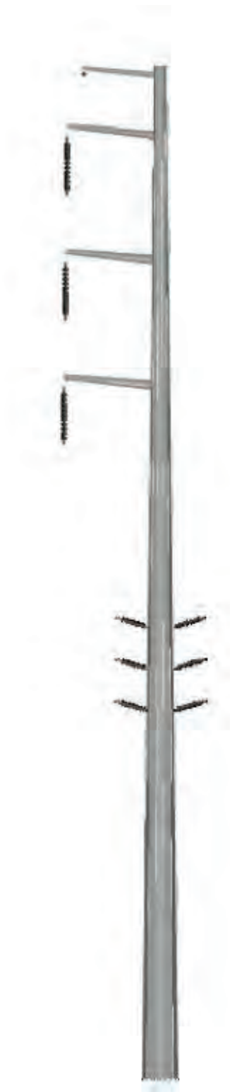
Single Circuit 230 kV Single-Pole, Vertical-Davit-Suspension
