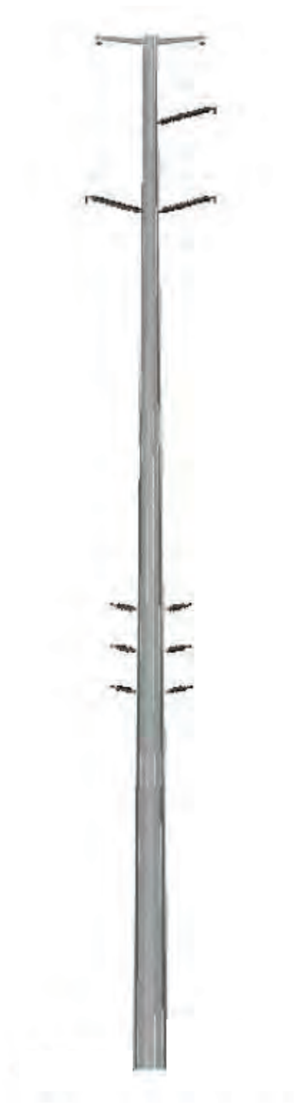
Single Circuit 230 kV Single-Pole, Delta-Post
