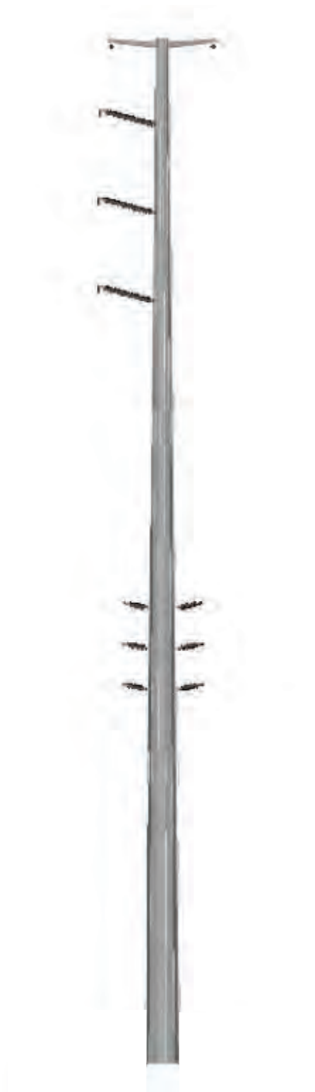
Single Circuit 230 kV Single-Pole, Vertical-Post
