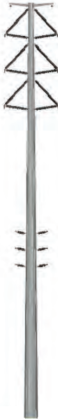
Double Circuit 230 kV Single-Pole, Braced-Post
